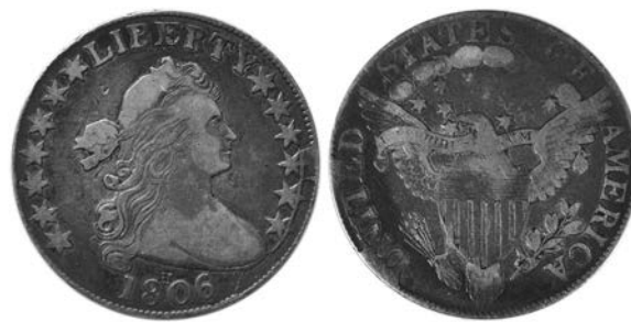
Image: This 1806/5 Draped Bust half dollar (attributed as Overton 104b and Tompkins T-1 varieties) indicates the problem of working die failure at the early Mint, with a large obverse die crack, and reverse edge cuds. (Author's collection.)
