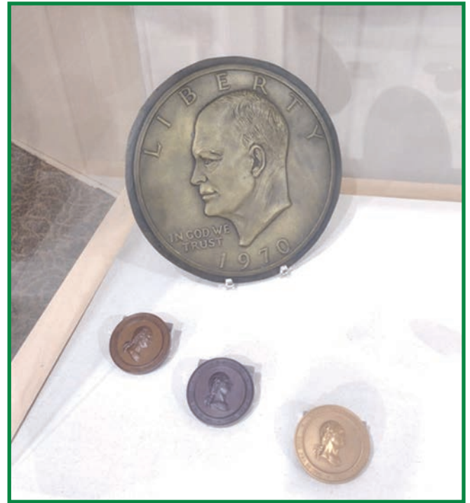
One of the original galvanos used to make Eisenhower Dollars. Author's photo from Summer Seminar 2024. This is part of "The Medal in America" display at the ANA Money Museum.
